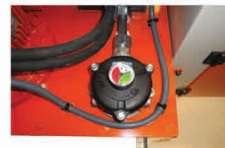
Duble oil filters; suction and return; oil pollution indicator
