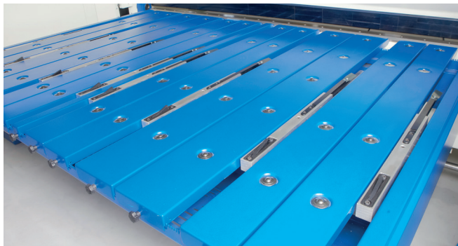
2000 / 3000 / 4000 mm motorized back gauge system and sheet support table with ball casters.
