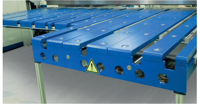
L shape back gauge system (metal or with brushes).
