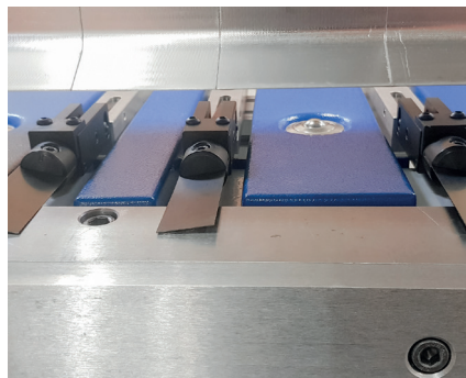
Solid lower beam tool with feather grooves
