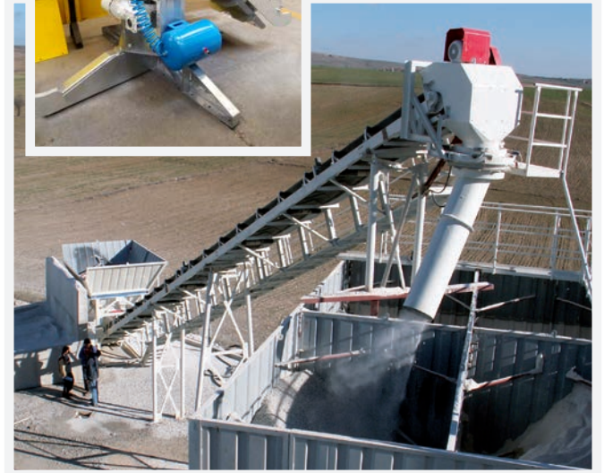
Bottom drive new distribution system with pneumatically activated flap
