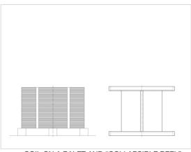
COIL ON A PALET AND "COLLAPSIBLE REEL" READY FOR ANOTHER WINDING OPERATION
