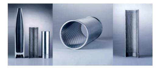
Gun barrel production using Repkon Free Flowforming Technology presents a superior alternative to conventional manufacturing techniques such as Single Point or Multipoint Broach Cut Rifling, Button Rifling, Hammer Rifling and Electro Chemical Machining etc.
