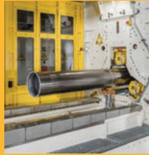
The new RFFM Series now brings about multi rollers for the production of dimensionally precise, tubular hollow work pieces. The fixed roller housing of the CNC controlled machine can be equipped with three, four, five or six rollers depending upon customer requirements, including **extremely large diameter** part productions!
