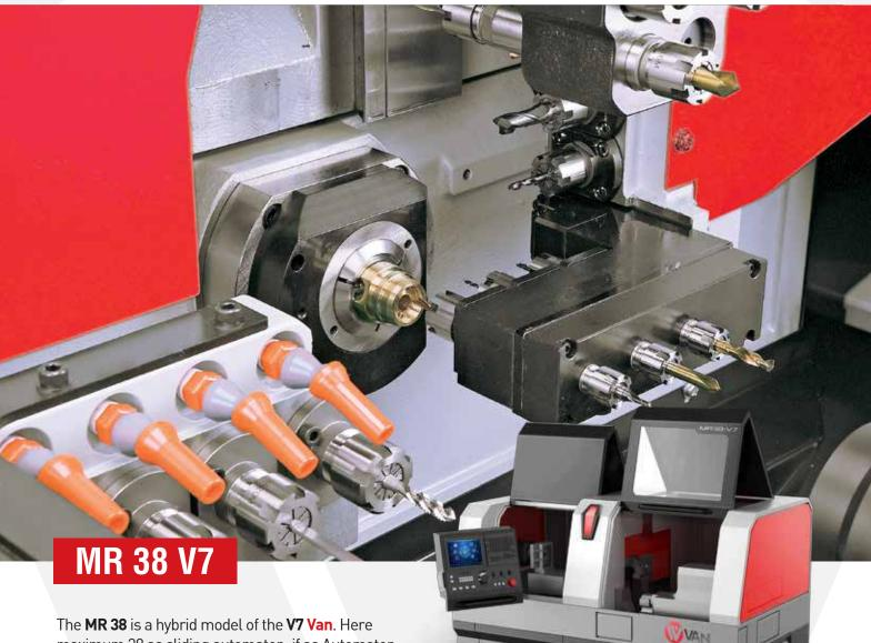
The MR 38 is a hybrid model of the V7 Van. Here maximum 38 as sliding automaton, if as Automaton raw material up to 42 mm max diameter you can manipulate. Machine 11 kW main spindle motor almost a show of strength to your opponents with strength references Especially the need of the automotive industry 42 mm diameter with this machine we are able to solve.
