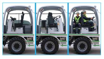
ROPS and FOPS level 2 certified closed operator cabin with 180  $^{\circ}\textsc{pivoting}$  operator's seat
