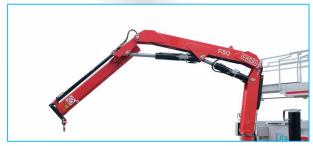
46 kNm lifting capacity, 4.9 m crane
