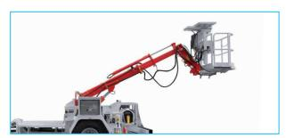
1590 x 790 mm, 500 kg lifting capacity basket
