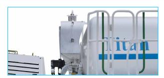
5.6 m³ concrete yield 220 l stainless steel admixture tank (optional)
