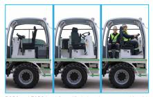
ROPS and FOPS level 2 certified closed operator cabin with  $180^{\rm o}{\rm pivoting}$  operator's seat
