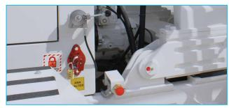
Locked type battery isolator switch
