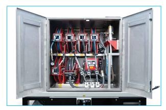
Fuel/oil transfer hoses with reels and flow meters
