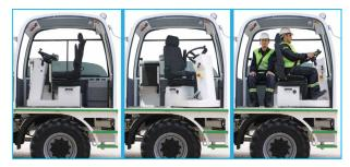
Closed cabin with 180° pivoting operator seat and ROPS & FOPS Level 2 certification
