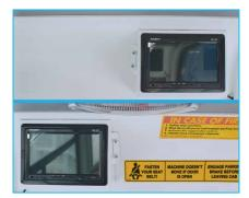
Rear view camera and LCD screen in operator cabin
