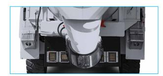
Hydraulically controlled shutter and chute
