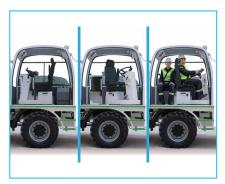
ROPS and FOPS level 2 certified closed operator cabin with 180° pivoting operator's seat
