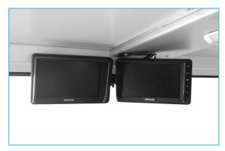
Rear view camera and LCD screen in operator cabin
