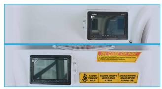
Rear view camera and LCD screen in operator cabin
