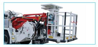
$1590 \times 790$  mm, 500 kg lifting capacity basket
