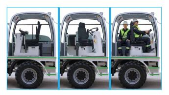
ROPS and FOPS level 2 certified closed operator cabin with 180° pivoting operator's seat
