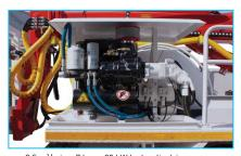
3.5 m³/min – 7 bar – 23 kW hydraulic driven screw compressor
