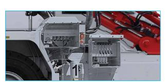
Control panel for manipulator and stabilizers
