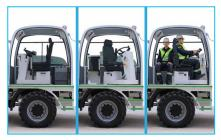
ROPS and FOPS level 2 certified closed operator cabin with 180° pivoting operator's seat
