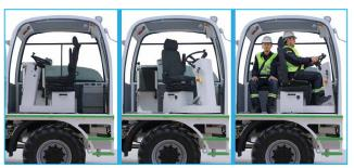
ROPS and FOPS level 2 certified closed operator cabin with 180° pivoting operator's seat
