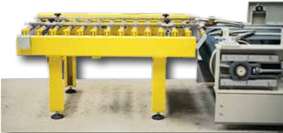
Motorlu ilave. Motorized roller conveyor.
